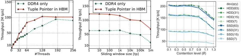
(a) Throughput with varying thread count (10k window size). (b) Throughput with varying window size (64 threads). (c) LSM-tree with varying devices (dev) and ad-hoc queries (qry).
