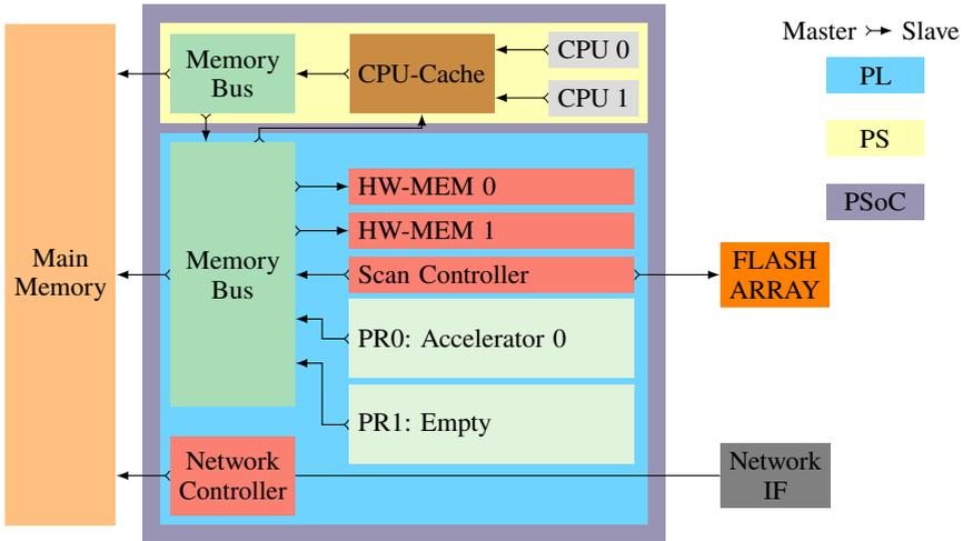
Fig. 1: Architecture of a ReProVide platform. Next to statically implemented IPs such as the *Network Controller*, *Scan Controller*, and heterogeneous (on- and off-chip volatile and non-volatile) memory resources, also partially reconfigurable areas are shown (*PR0*, *PR1*). These areas are reconfigured during runtime, loading presynthesized hardware modules. Additionally, a Processing System (PS) containing a dual core ARM-based processor is contained on the SoC.
