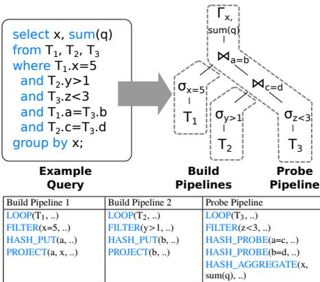
Fig. 2: Segmentation of example query into pipeline programs.
