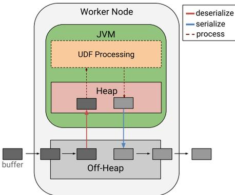
Fig. 1: Current UDF processing method.
