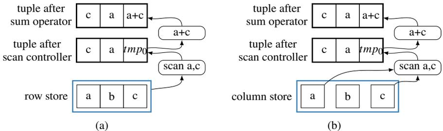
Fig. 2: A tuple  $(a, b, c)$  being processed according to the query `SELECT c, a, (a+c)`; using a row-oriented storage (a) and a column-oriented storage (b). First, the scan controller produces a new tuple with placeholders and the requested order of attributes. In the next step, the *sum* function is applied to this tuple and the result is written to the previously created placeholder field ( $tmp_0$ ).
