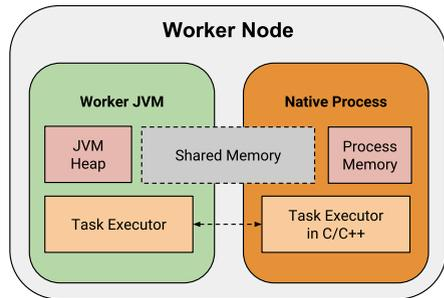
Fig. 2: UDF computation offloading.
