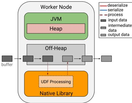
Fig. 3: Off-Heap data exchange.
