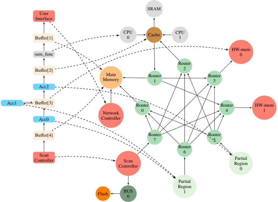
Fig. 5: Problem graph (left) and its binding to the architecture graph of a heterogeneous architecture such as the ReProVide platform depicted in Fig. 1. The communication resource *BUS0* models the half duplex connection between the *Flash*-Memory and the *Scan Controller*.
