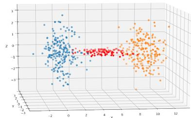
Fig. 1: The red points cause a density-connection between the intentional two clusters and thus form a chain.
