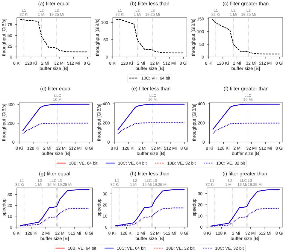
Fig. 5: Measured throughput of VH and engine as well as the speedup obtained by the VE of different Bitweaving-H operations executed using one thread.
