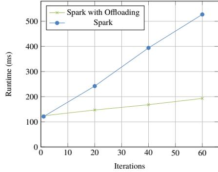
Fig. 7: Compute-heavy UDF in Spark
