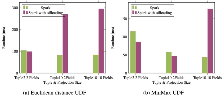
Fig. 8: Computation Offloading prototype evaluation.
