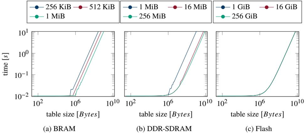
Fig. 8: Execution time for two accelerators scheduled on the same partial reconfigurable area to process tables of different sizes. A buffer is allocated for exchanging data between both accelerators. Reconfiguration between accelerators is performed as soon as all tuples are produced in/consumed from the buffer. Per memory type, the execution time for different sizes allocated for this buffer is depicted.
